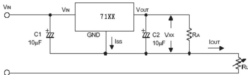
$$I_{OUT} = V_{XX}/R_A + I_{SS}$$
