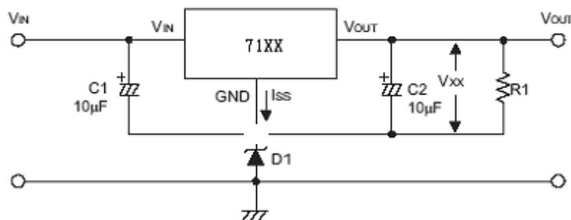
$$V_{OUT} = V_{xx} + VD1$$
